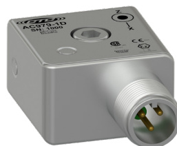
AC979 Nonincendive, intrinsically safe, X and Z axes, 100 mV/g, ±10%
