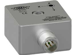
TXFA331-VT Premium, piezo velocity and temperature output, 500 mV/in/sec, 10 mV/°C, ±5%
