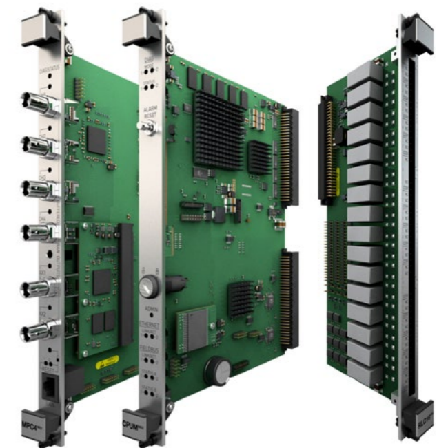
Our 2nd generation VM600 platform introduces (L to R) the MPC4 Mk2 , CPUM Mk2 , and RLC16 Mk2 modules along with companion I/O cards.
