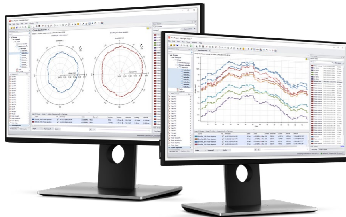
Figure 6: The VibroSmart and VM600 platforms are fully supported by VibroSight software including the diagnostic rule box “decision support” capabilities (top) and the specialized plot types such as air gap (bottom) unique to hydro machines.
